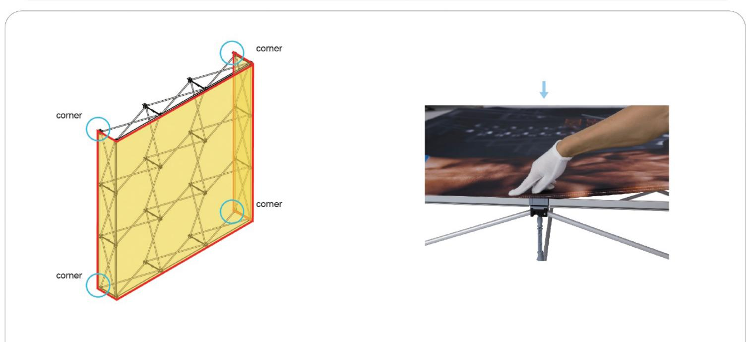
4. Slide the graphic into channel bar. (The corner first, then the middle of graphic)
