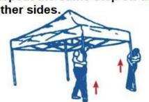
2B. Grab the scissor bars that are connected to the middle leg, lift them up and step backwards until the tent is fully extended. Be cautious not to get pinched by the frame.
