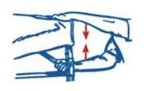
2A. Grab the bottom of the scissor bar, lift it up and step backwards until the tent is fully extended. Be cautious not to get pinched by the frame (for 10x20 tent, see 2B).
