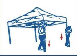
2. Release the auto slider by pushing the push-pin and pulling it down. Repeat the same step on the other sides.
